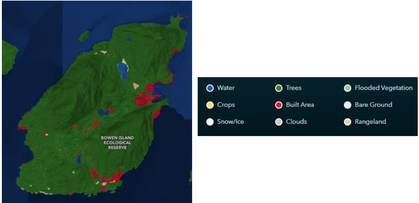
Figure 2 ESRI Sentinel 2 Land cover explorer using 10 m imagery but only nine land cover classes.
